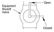
Figure 42 - Equipment Shutoff Valve
